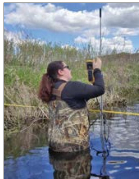
Jaxsyn Olson collects a stream sample using a Van Dorn (top). Julia McGee uses a FlowTracker for a streamflow measurement (bottom).
